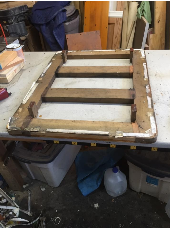
Above: Regulator top, upside-down on workbench, as seen from the inside. Ribs and bottom removed.
