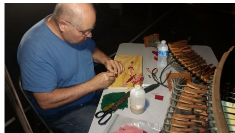
Jeff Slabaugh works on restoring pneumatics for the combination action.
