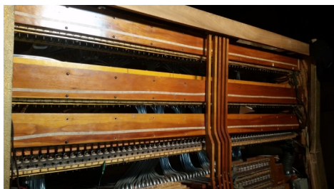
Back of organ console, showing the "blow boxes" for the combination action.
