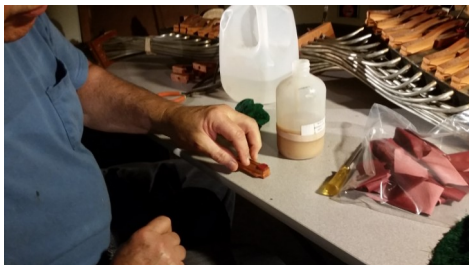
Jeff Slabaugh is waiting for glue to dry on newly-releathered pneumatics.
