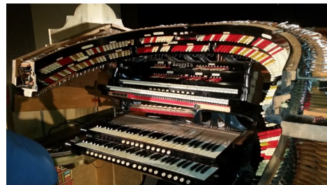
The console is opened up so that the piston rail can be worked on.
